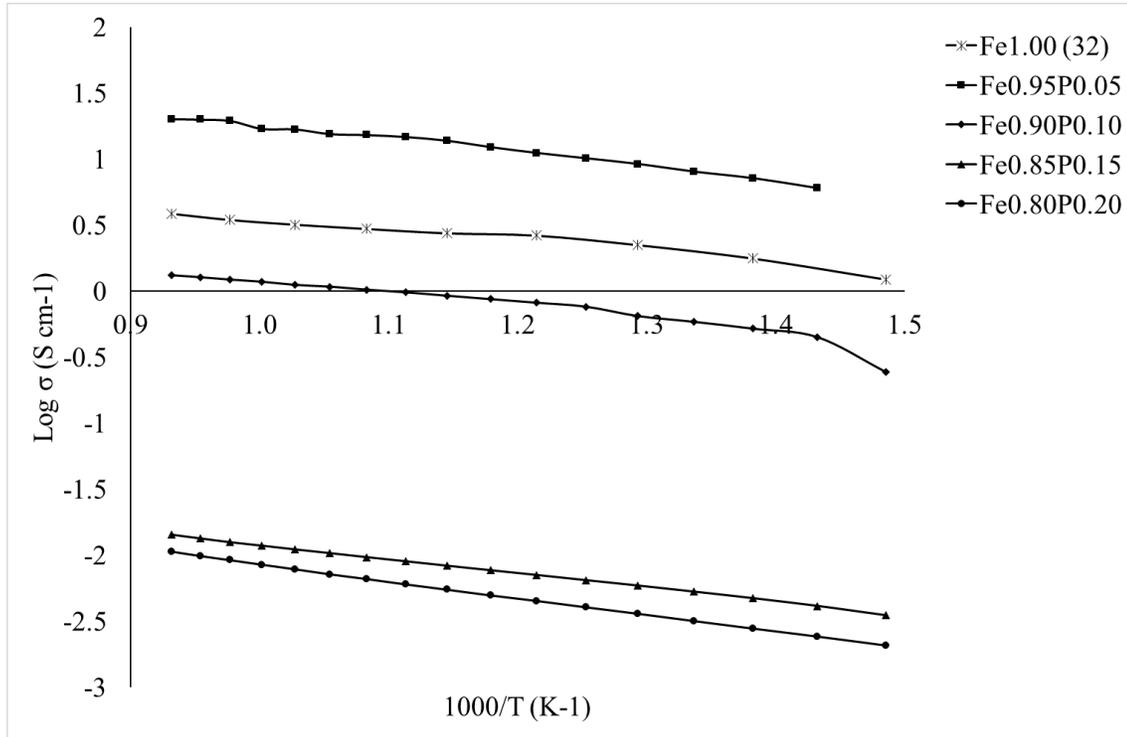
Figure 6: Plot of  $\log \sigma$  versus  $1000/T$  for  $\text{Sr}_2\text{MnFe}_{1-x}\text{P}_x\text{O}_{6-\delta}$
