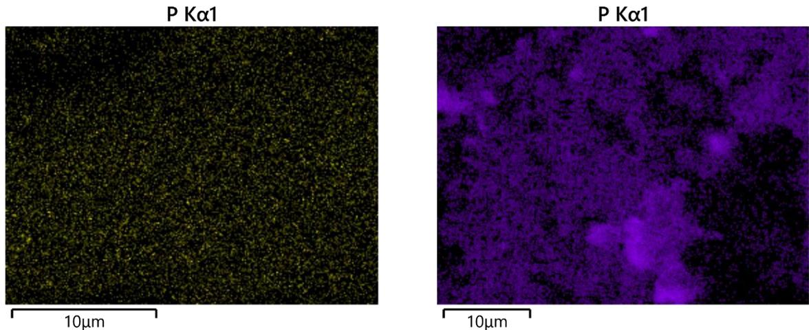
Figure 5: Energy-dispersive X-ray spectroscopy imaging of P ( $K\alpha_1$ ) content (left)  $\text{Sr}_2\text{MnFe}_{0.95}\text{P}_{0.05}\text{O}_{5.41}$  and (right)  $\text{Sr}_2\text{MnFe}_{0.80}\text{P}_{0.20}\text{O}_{5.29}$
