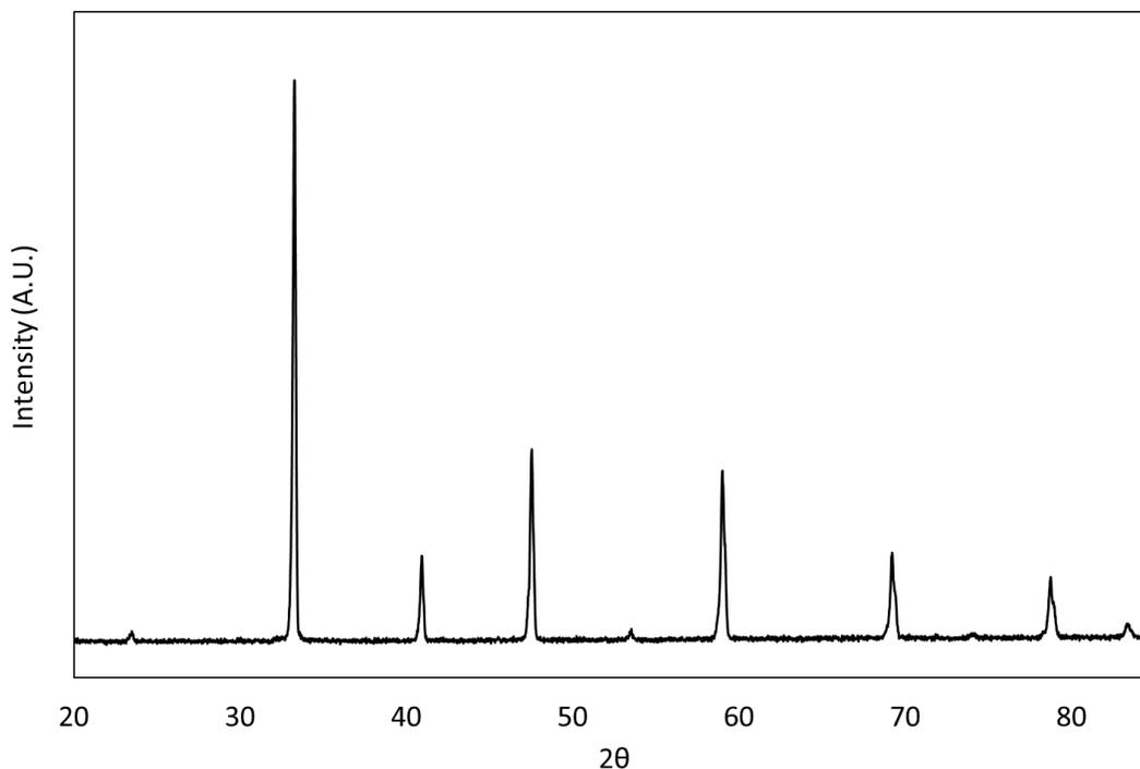
Figure 1. Powder X-ray diffraction data of Sr<sub>2</sub>MnFeO<sub>6-δ</sub> showing formation of a single phase cubic perovskite.
