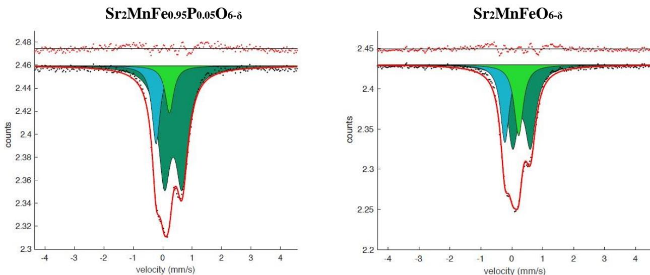
Figure 4. <sup>57</sup>Fe Mössbauer spectra for  $\text{Sr}_2\text{MnFe}_{0.95}\text{P}_{0.05}\text{O}_{6-\delta}$  and  $\text{Sr}_2\text{MnFeO}_{6-\delta}$  at 298 K
