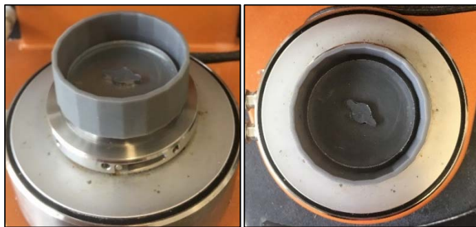
435 Figure 2 – Photographs of 3-D printed base plate (tribometer cell) for holding the PDMS disc.
