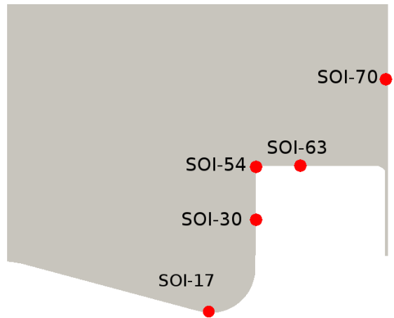
Figure 1: Cross section of the cylinder showing a central plane of the sector mesh. Approximate spray impingement locations after half injection duration for all injection cases are marked with red dots.
