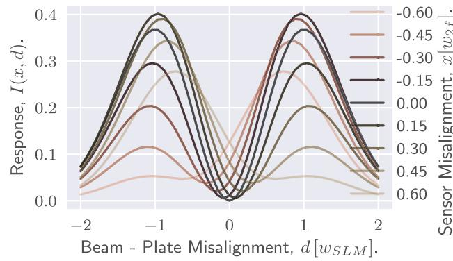
**Fig. 7.** Ideal response of alignment MODAN to a relative misalignment between the beam and the phase-pattern, for several light-sensor positions. This is computed using Eq. (18), with  $a_0^H, a_1^H$  from 19, 20 and inter-modal phase difference  $\phi_0 - \phi_1 = \frac{\pi}{4}$ .
