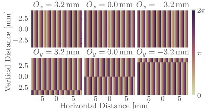
**Fig. 4.** Phase-patterns with various software offsets. Upper patterns are  $T_{10}^{PO}$  and lower pattern are  $T_{01}^{PO}$ . The grating period has been increased from  $80 \mu\text{m}$  (10 pixels) which was used in the experiment, to  $1536 \mu\text{m}$  and the number of pixels decreased by a factor 10 in both directions, to provide a legible figure.
