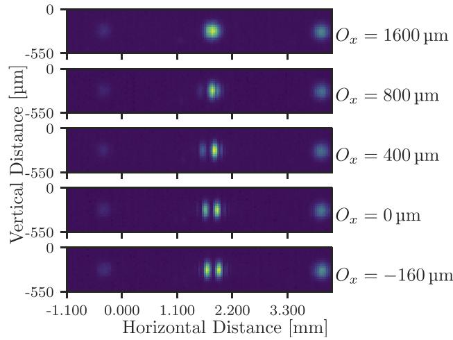
**Fig. 5.** Camera images for several phase-pattern offsets.  $O_x$  is the phase-pattern offsets with respect to the SLM. The central spot is the first diffraction order, with the specular and the second diffraction orders either side.
