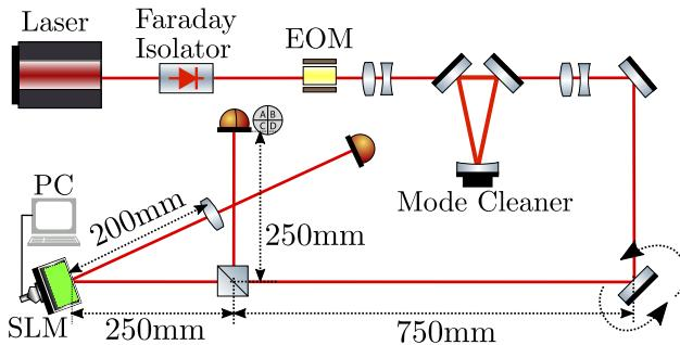
**Fig. 2.** Simplified Experimental Layout. The light is first filtered through an optical cavity to generate a high purity HG00 mode. A pair of steering mirrors then add controlled misalignment to the beam. The light is split between the MODAN under test and a witness QPD. The SLM is configured to display phase-pattern,  $T(x, y)$  and works in reflection. Extraneous lens, waveplates and mirrors are not shown.
