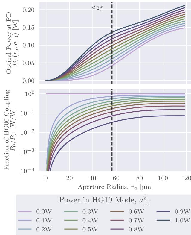
**Fig. 9.** The upper plot shows the total optical power on the light-sensor as a function of aperture radius, for 1W total power and different amounts of HG10 power. The lower plot shows the fraction of this light which is crosstalk from the HG00 mode. The parameters used were:  $\lambda = 1064$  nm,  $f = 0.2$  m,  $b_{10} = w_{\text{SLM}} = 1.2$  mm,  $a_{00}^2 = 1 - a_{10}^2$ .  $w_{2f}$  is given by Eq. (16).
