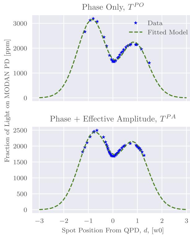
**Fig. 8.** A steering mirror was used to scan the relative alignment between the incident light and a static phase-pattern on the SLM, a QPD was used as a witness sensor. Data could only be obtained in the region  $|d| < 1$  due to the limited range of the QPD. The photo-diode offset, computed during the fit, has been added to both the data and the model. The upper and lower plots show the response for phase-pattern described by Eqs. (5) and (7), respectively.
