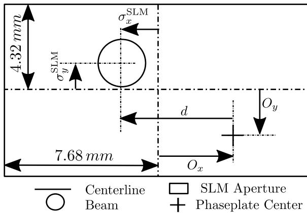
**Fig. 3.** SLM Geometry to scale. The solid circle illustrates the point at which the power of the spatially fundamental beam falls to  $1/e^2$  of peak intensity.  $\sigma_{x,y}^{SLM}$ , describes the position of the beam with respect to the SLM,  $O_{x,y}$  describes the offset in software between the phase-pattern center and the SLM center and  $d$  describes the relative  $x$  offset between the phase-pattern origin and the beam.
