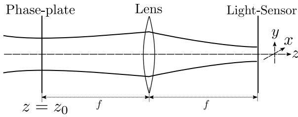
**Fig. 1.** Optical Convolution System. The light is incident on a DOE resulting in the field just after the DOE being,  $U(x, y) = U_{\text{in}}(x, y)T(x, y)$ . The light propagates a distance of  $2f$  to a light-sensor (we use photodiode masked by a pinhole), with a lens of focal length  $f$  placed half way between the sensor and the DOE.
