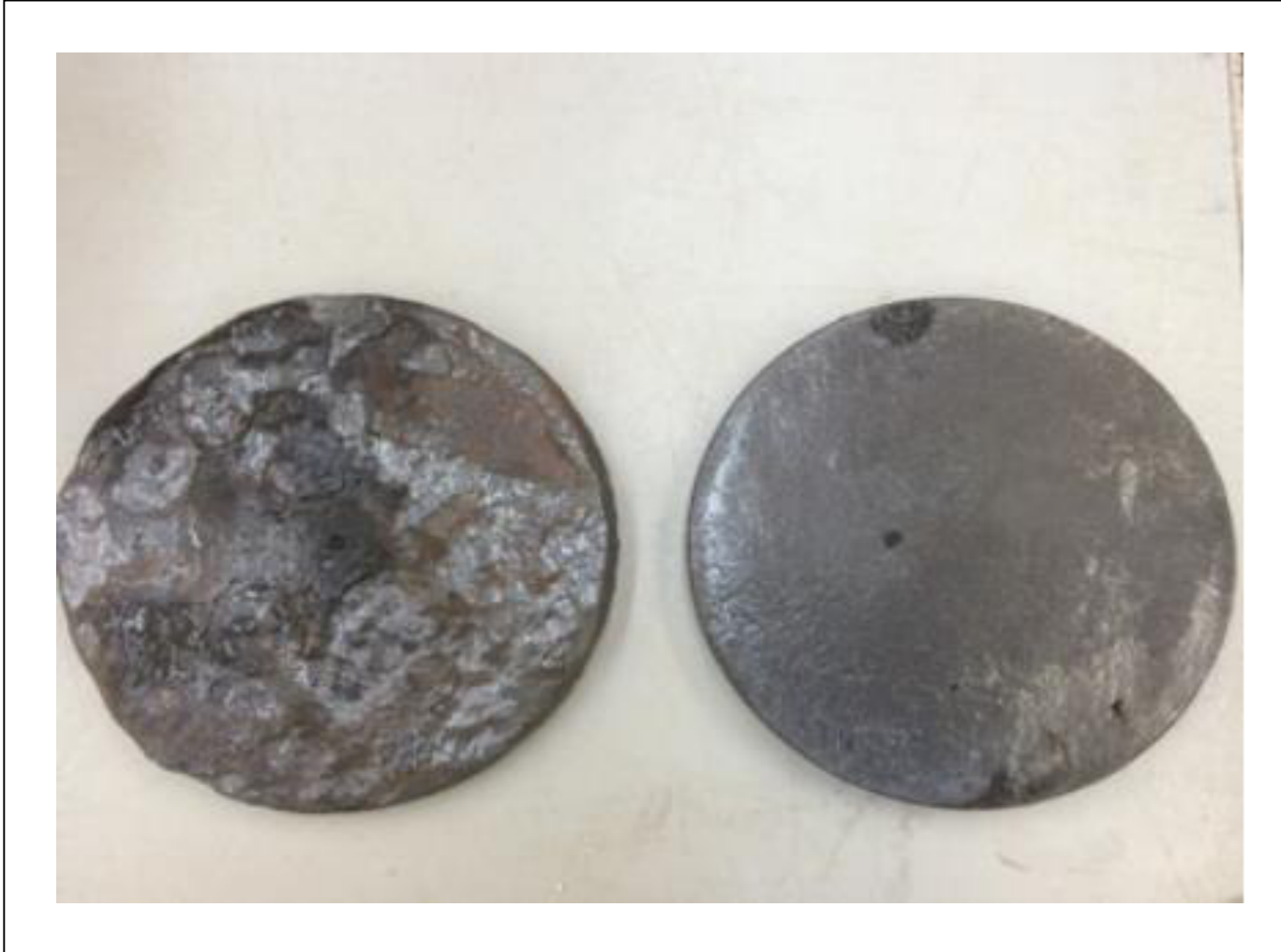
Figure 10: Cast iron discs removed at the end of the 3-months test for the Oxford Clay (left) and the Kaolin Clay (right)
