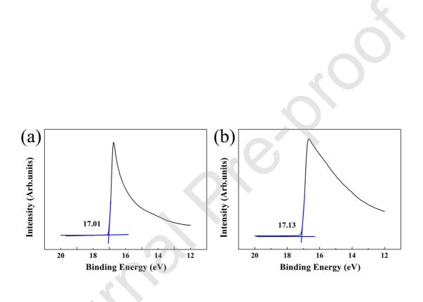
10. Fig. 10. High-binding-energy regions of UPS spectra of (a) pure  $In_2O_3$  nanofibers and (b)  $Zn-In_2O_3$  composite nanofibers.
