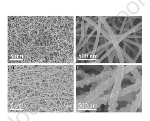
2. Fig. 2. SEM images of (a) pure In<sub>2</sub>O<sub>3</sub> nanofibers and (c) Zn–In<sub>2</sub>O<sub>3</sub> composite nanofibers; (b) and (d) are the corresponding high magnification SEM images of pure In<sub>2</sub>O<sub>3</sub> nanofibers and Zn–In<sub>2</sub>O<sub>3</sub> composite nanofibers, respectively.
