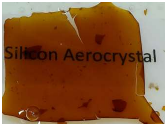
Figure 1. Optical images of Si wafer (thickness of 650 microns) and membranes of varying porosity but constant thickness of 55 microns. (a) 0% (bulk Si) (b) 84% (c) 87% (d) 90% (e) 93%. The images (b-e) are from an anodized membrane of 81% porosity that was etched in 10% ethanoic HF for increasing periods of 1, 2, 3 and 5 hours, respectively.
