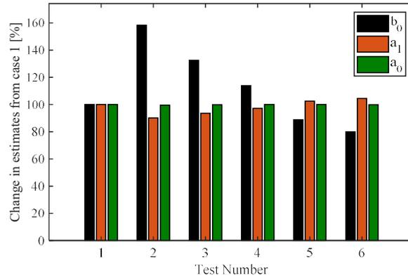
Fig. 6 Case 1: Three estimates of inertia are uncorrelated ( $<0.8$ )
