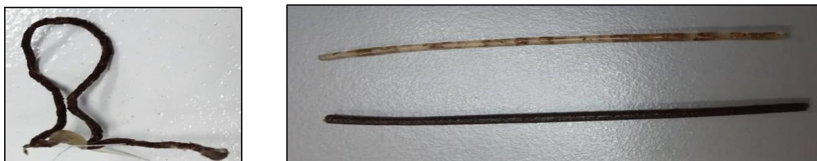
Figure 12. (Left) Flushed fibers after the degradation out of extrusion die and (Right) Successful extrusion of 5wt% Untreated PCSPC (bottom) and PCFC (top) composite filament.
