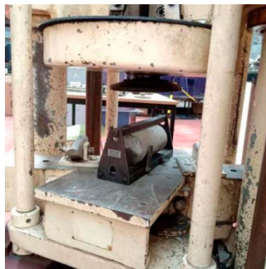
Figure 6. Splitting tensile test setup.
