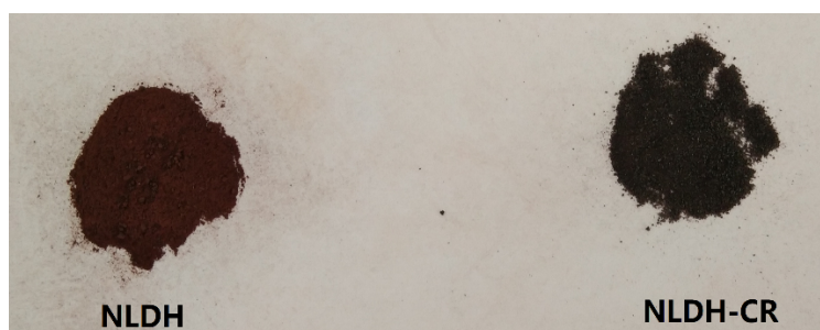
Fig. S7 Picture of NiFe 2 O 4 /ZnCuCr-LDH (NLDH) before and after CR removal
