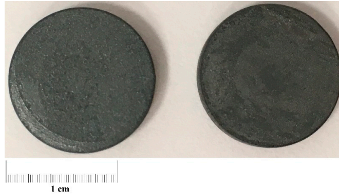
Figure 6. Photo of the 47ND alloy samples without ( left ) and with ( right ) modification of the surface.
