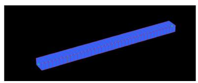
**Figure 1.** Finite element analysis for modelling of an FFU composite beam in the free-free condition **Table 1.** Engineering properties utilized in the dynamic modelling [28]
