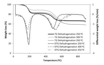
**Fig. 7** TGA of the used catalyst after 6 h experiment at 250, 300 and 350 °C under induction heating at pressure 18 barg, LHSV 0.75  $h^{-1}$ , CTSBR 70% v/v and gas flow rate of 200 mL min<sup>-1</sup> (N<sub>2</sub>)
