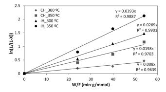
**Fig. 10** First-order kinetic plot using Eq. 1 for IH and CH at 300 and 350  $^{\circ}$ C at pressure 18 barg, LHSV 0.75 h<sup>-1</sup>, CTSBR 70% v/v and gas flow rate of 200 mL min<sup>-1</sup> (N<sub>2</sub>)
