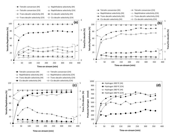
Fig. 9 Tetralin dehydrogenation conventional heating (CH) against induction heating (IH) at **a** 300 °C, **b** 350 °C, **c** 380 °C and **d** produced hydrogen due to naphthalene formation at pressure 18 barg, LHSV 0.75  $h^{-1}$ , CTSBR 70% v/v and gas flow rate of 200 mL min<sup>-1</sup> (N<sub>2</sub>)
