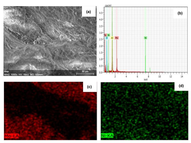
Fig. 3 NiMo/Al<sub>2</sub>O<sub>3</sub> catalyst morphology. a SEM micrograph, b EDS, c Mo metal mapping and d Ni metal mapping
