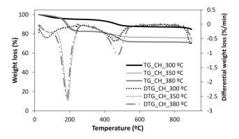
Fig. 11 TGA of the used catalyst after 6 h experiment at 300, 350 and 380 °C under conventional heating at pressure 18 barg, LHSV  $0.75~h^{-1}$ , CTSBR 70%~v/v and gas flow rate of  $200~mLmin^{-1}~(N_2)$
