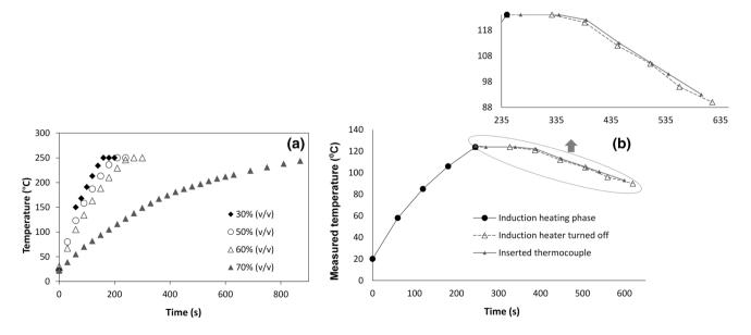
Fig. 4 Catalyst bed temperature  $\mathbf{a}$  as a function of CTSBR (v/v) and  $\mathbf{b}$  the influence of magnetic field and eddy current on the temperature reading of the thermocouple at 70% CTSBR
