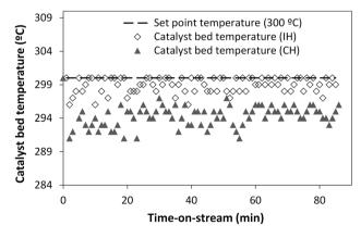
**Fig. 8** Catalyst bed temperature for IH and CH at temperature 300 °C, CTSBR 70% (v/v), LHSV  $0.75~h^{-1}$ , pressure 18 barg and 200 mL min $^{-1}$  nitrogen flow
