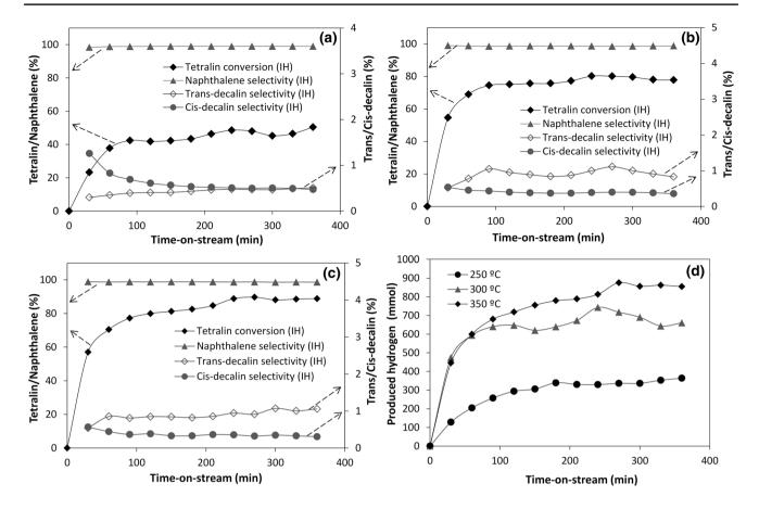
Fig. 5 Tetralin dehydrogenation under induction heating at  $\bf a$  250 °C,  $\bf b$  300 °C,  $\bf c$  350 °C and  $\bf d$  produced hydrogen at pressure 18 barg, LHSV 0.75 h<sup>-1</sup>, CTSBR 70% v/v and gas flow rate of 200 mL min<sup>-1</sup> (N<sub>2</sub>)
