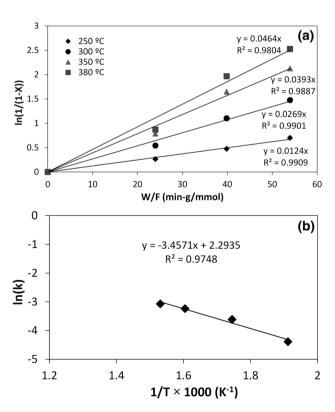
**Fig. 6** Tetralin dehydrogenation using Ni–Mo/Al<sub>2</sub>O<sub>3</sub> at 250, 300, 350 and 380 °C in the fixed-bed catalytic reactor with CTSBRs 35%, 50% and 70% (v/v), pressure 18 barg, LHSV 0.75 h<sup>-1</sup>, and gas flow rate of 200 mL min<sup>-1</sup> (N<sub>2</sub>): **a** first-order kinetic plot using Eq. 1 and **b** Arrhenius equation
