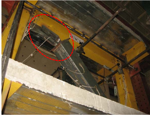
(a) Out-of-plane deformation of BRB in the 2nd story
