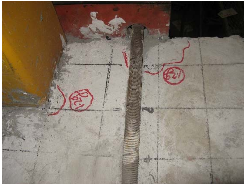
(a) Out-of-plane deformation of BRB in the 2nd story
