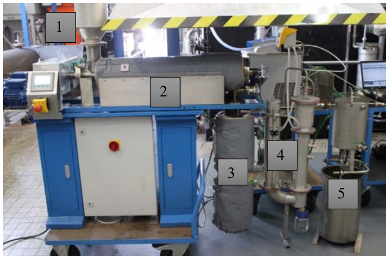
Figure 3. TCR ® 2 (Lab scale) – maximum capacity 2kg/hr. 1) feed hopper, 2) reactor, 3) post-reformer, 4) gas cooler/ condenser #1, 5) gas cooler/condenser#2
