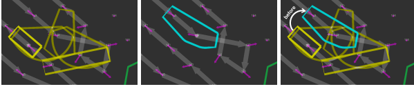
FIGURE 5. Coordinating two machines to avoid spatio-temporal overlap.
