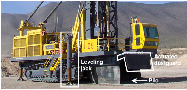
FIGURE 2. The actuated dust guard and leveling jacks are highlighted on an Atlas Copco Pitviper-271. After drilling, piles of excess material accumulate under the dust guard, which requires the machine to actuate the dust guard before navigating away from the target.
