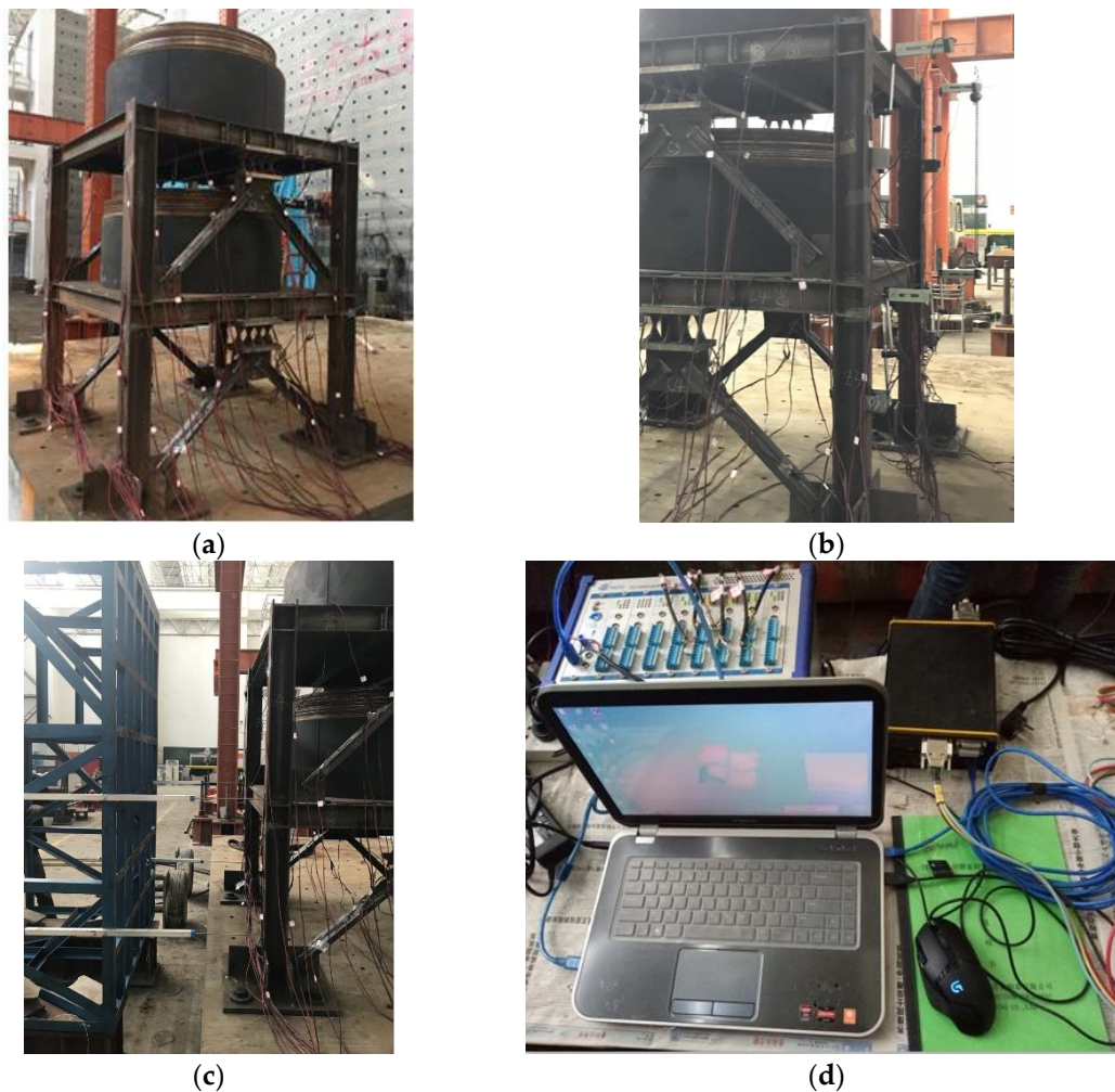
Figure 12. Measuring devices of the specimen. (a) Connection of strain gauges; (b) YHD sensors; (c) TST sensors; (d) data acquisition instrument.
