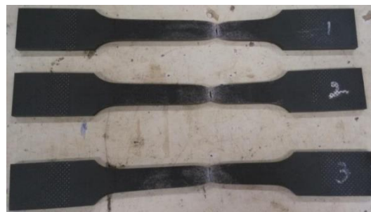
Figure 7. Fractured LYP steel coupons.
