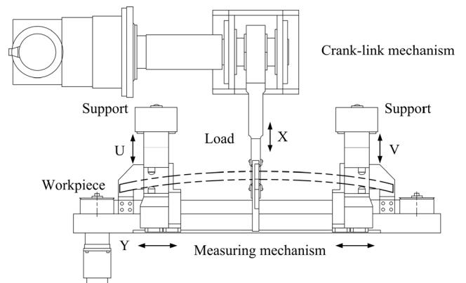
**FIGURE 4.** Straightening machine.
