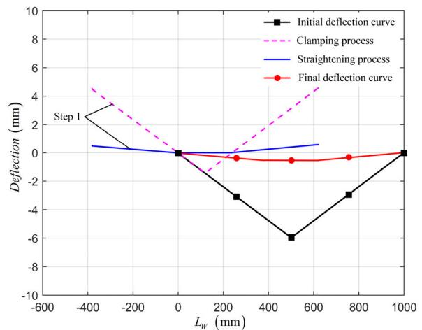
**FIGURE 12.** Theoretical results of the fine straightening stage for the single-arc deflection curve.
