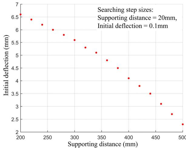
**FIGURE 3.** Deflection-distance distribution avoiding the unexpected deformation.
