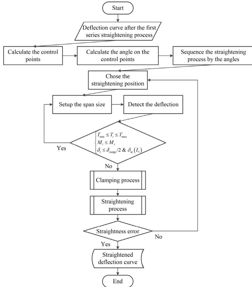
**FIGURE 10.** Flow chart for the fine straightening stage.
