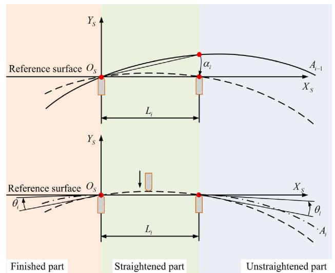
**FIGURE 9. Schematic for the clamping and straightening processes.**
