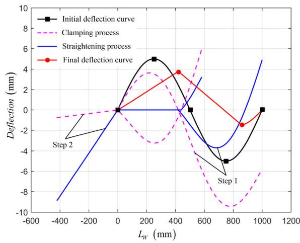
**FIGURE 14.** Theoretical results of the major straightening stage for the 'S'-shape deflection curve.**TABLE 4.** The parameters of the fine straightening stage for the 'S'-shape deflection curve.
