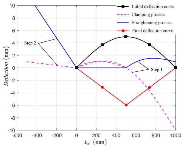
**FIGURE 11.** Theoretical results of the major straightening stage for the single-arc deflection curve.**TABLE 2.** He parameters of the fine straightening stage for the single-arc deflection curve.
