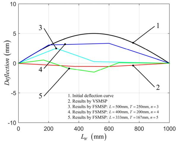
**FIGURE 13.** Comparison of theoretical results by VSMSP and FSVSP for the single-arc deflection curve.
