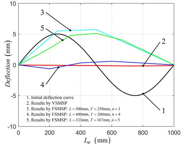
**FIGURE 16.** Comparison of theoretical results by VSMSP and FSVSP for the 'S'-shape deflection curve.
