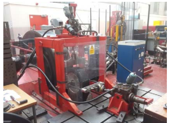
Figure 6. Laboratory Tire-Drum Testing Equipment.
