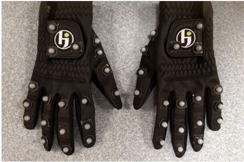
Figure 6: The motion capture gloves used in our study. Each glove has 19 markers, with finger markers being placed between joints. In the Glove condition, we receive global wrist positions and orientation along with the poses of fingers.
