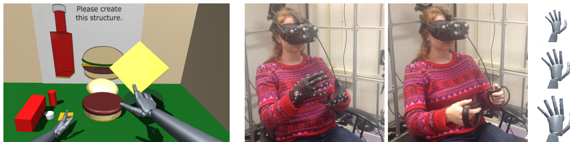
Figure 1: In our experiment, participants complete block stacking puzzles in virtual reality (left), controlling their avatar’s hands either with tracked gloves (middle, left) or with touch controllers (middle, right). The avatar’s hands are varied to fit the participant’s hands in size or to be 25% larger or smaller (right).
