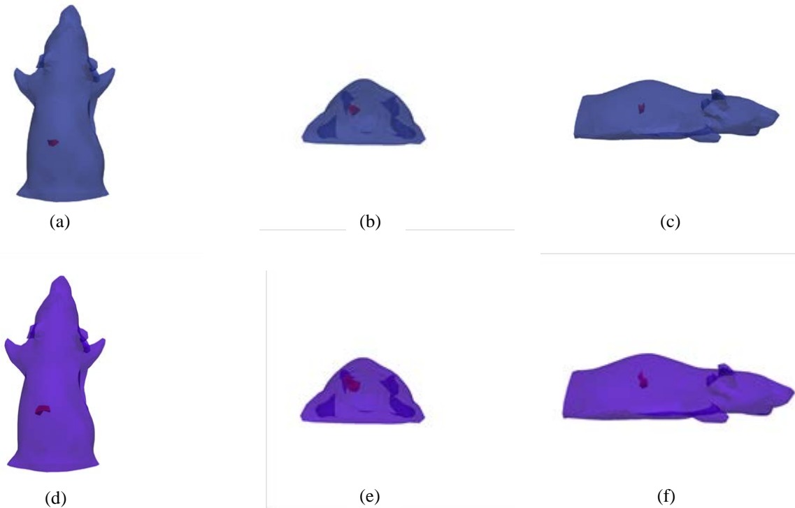
Figure 4: a-c) The ground truth location of the light source within the phantom. d-f) Tomographic reconstruction of the optical fibre light source within the mouse phantom.
