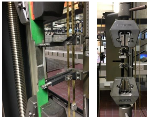
Figure 4: Material coupon testing apparatus and specimen fracture.
