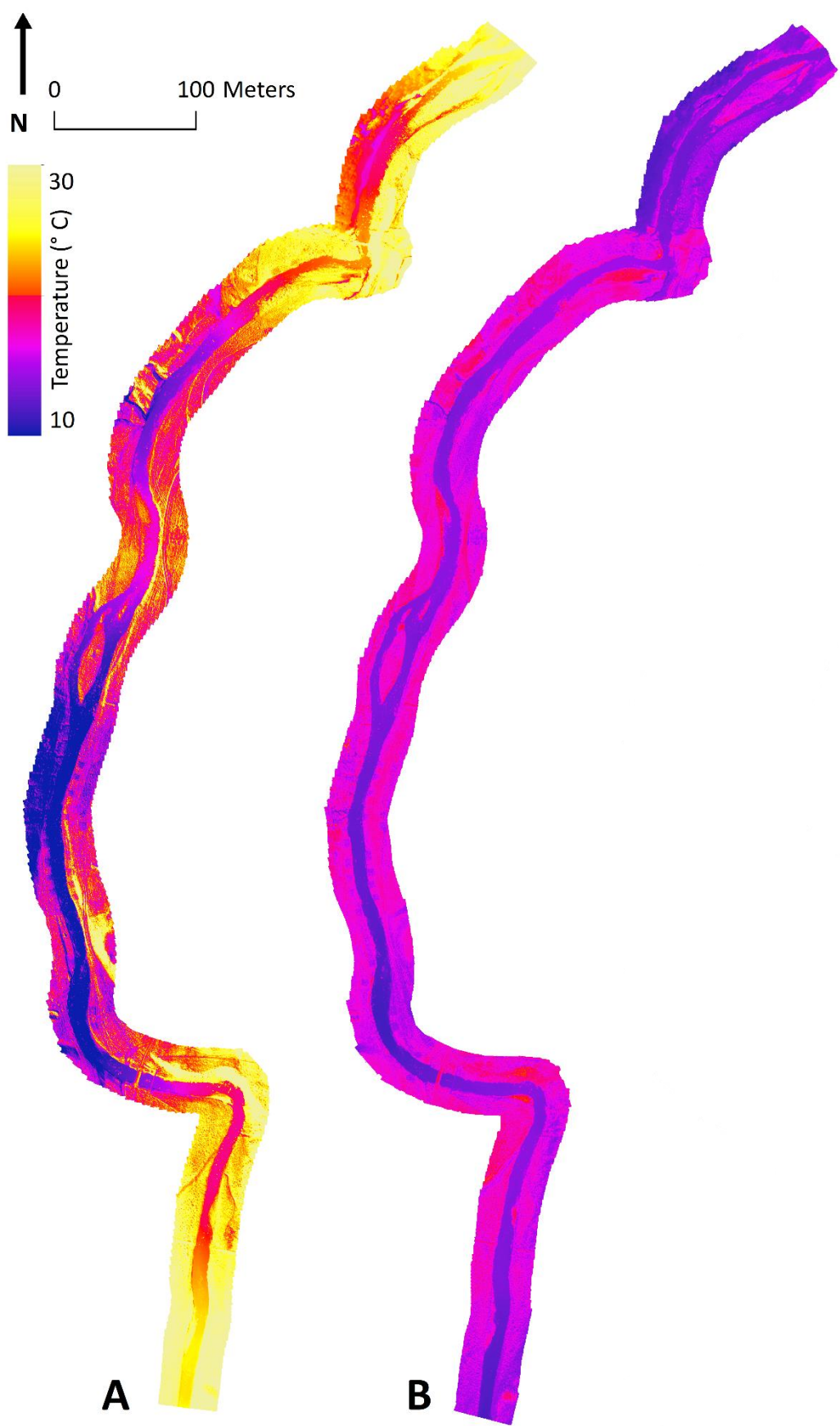
Figure 2. Drift-affected TIR image mosaics of Baddoch Burn showing (a) highest magnitude TIR drift observed over all flights (survey 3) and lowest magnitude TIR drift observed (survey 8). For more details on magnitude of drift, see Table S2.
