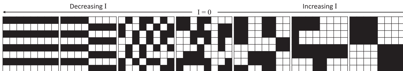
Fig. 1. Schematic diagram showing images containing equal numbers of black and white pixels. The central image is a random distribution of black and white pixels giving a Moran's I of 0, the images left of the center having more alternating black and white pixels and lower, more negative values of Moran's I and the images right of the center show more clustering and higher, more positive values of Moran's I .
