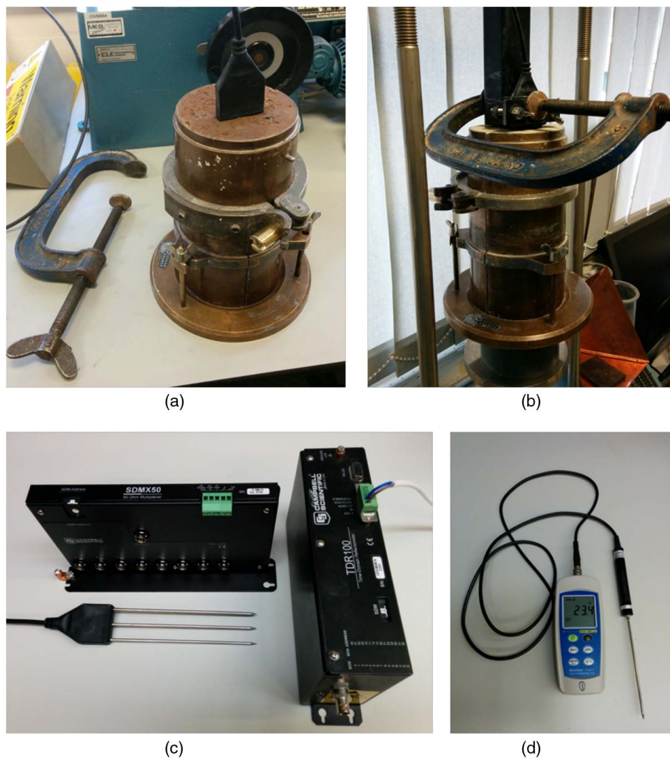
Fig. 3. (a) TDR probe inserted in a compaction mold; (b) clamp used to facilitate probe insertion in stiffer soils; (c) TDR equipment; (d) temperature sensor
