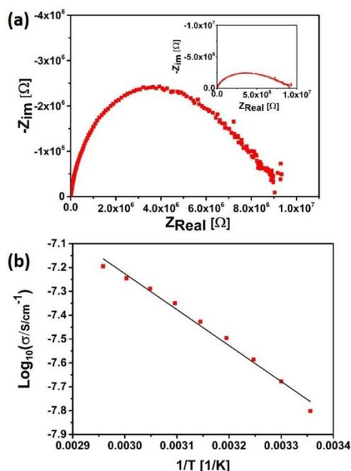
Figure 4: (a) Nyquist and (b) Arrhenius plot for temperature dependent total electrical conductivity of BaCoO<sub>2+ $\delta$</sub>  sample.
