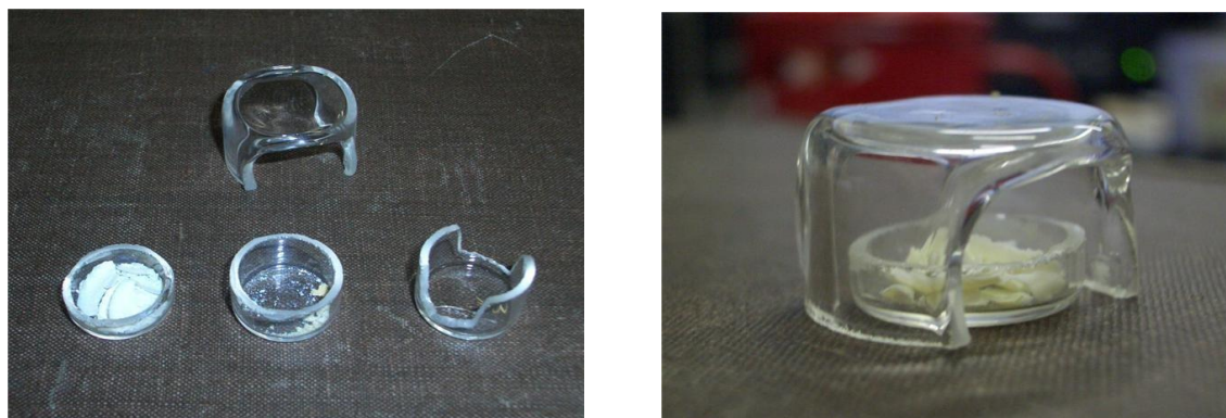
Figure 5. (a) The sample pans and the cover (b) Assembled pan and cover
