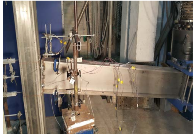
Fig. 4: General arrangement of experimental setup and instrumentation.
