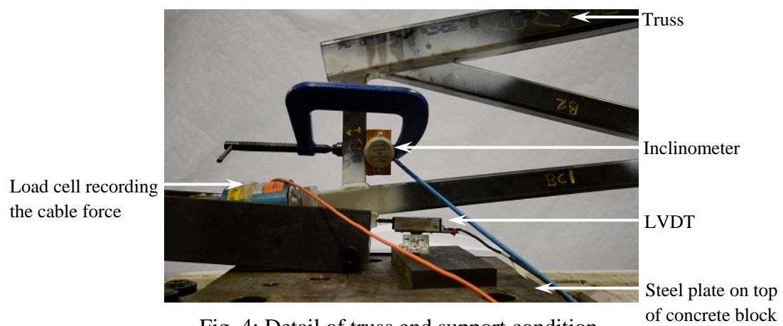
Fig. 4: Detail of truss end support condition.
