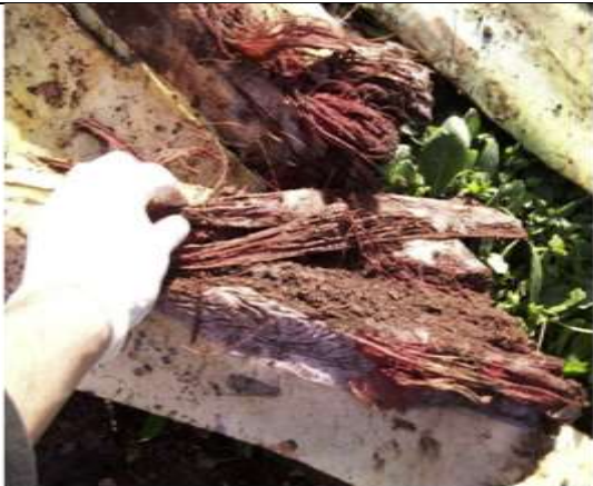
Fig. 3 (a). Extraction of fibers from the ground when the plant is buried (Bezazi et al., 2014). (Reproduced with permission from Elsevier, License Number- 4443450240953)
