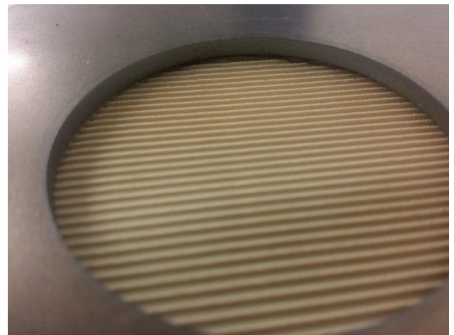
Figure 2 A single wafer sample in the holder.
