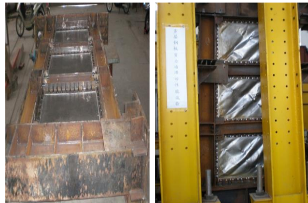
(a) Before loading (b) Ultimate deformation
