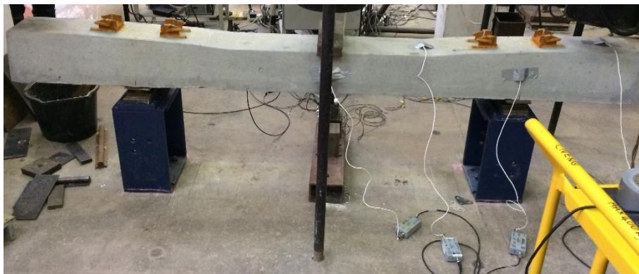
Fig. 2. Railway concrete sleeper placed on steel supports for three-point bending procedure.
