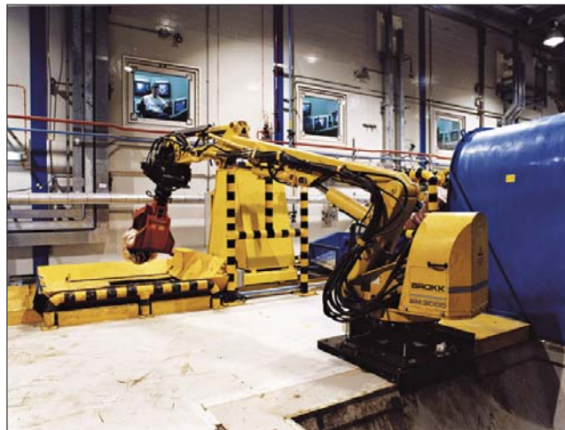
Fig. 1. A BROKK robot, equipped with a gripper, being used for a pick and place task at the Sellafield nuclear site in UK. This robot has no sensors for measuring joint angles, and so must be directly controlled by a human operator, who pushes a separate switch for each joint and judges the robot's pose by eye. The human operator can be seen controlling the robot from behind a 1.6m thick lead glass window which shields against radiation. For more examples, refer to www.sellafieldsites.com/solution/decommissioning/ .
