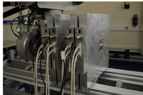
FIG. 2. The PRaVDA silicon tracker setup on an optical bench situated in the proton vault at iThemba LABS. The phantom is situated in the spacing that can be seen between the front and back pair of tracking units.
