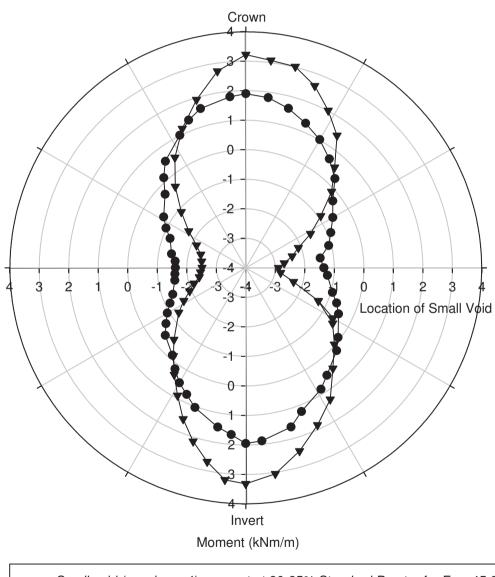
Small void (specimen 4) moment at 80-85% Standard Proctor for  $F_{H} = 45.9 \text{ kN/m}$ Intact soil (specimen 6) moment at 90-95% Standard Proctor for  $F_{H} = 45.9 \text{ kN/m}$
