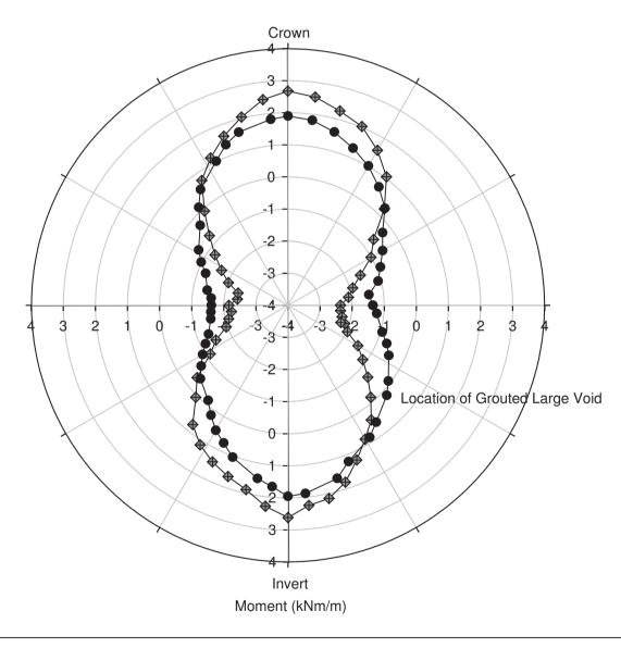
Grouted large void (specimen 7b) moment at 90-95% Standard Proctor for F<sub>H</sub> = 45.9 kN/m
