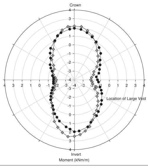
Large void (specimen 7a) moment at 90-95% Standard Proctor for  $F_{H} = 45.9 \text{ kN/m}$ — Intact soil (specimen 6) moment at 90-95% Standard Proctor for  $F_{H} = 45.9 \text{ kN/m}$
