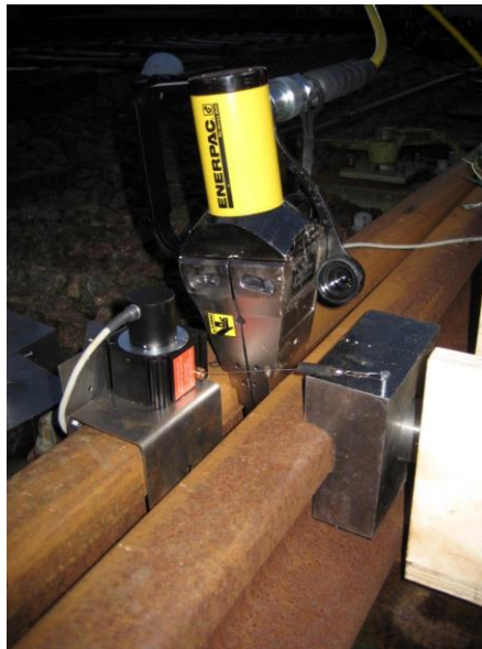
Figure 7. The wedge spreader used to simulate the run-through
