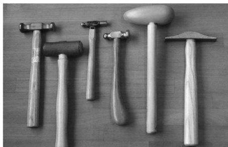
Fig. 5 Examples of jewellers' hammers: (from left) planishing, rawhide, ballpeen, chasing, bossing, forging
