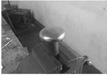
Fig. 4 A metal form (source: http://userblogs.ganoksin.com/primitive/2011/01/17/manufacturing-hammered-sheet/ )
