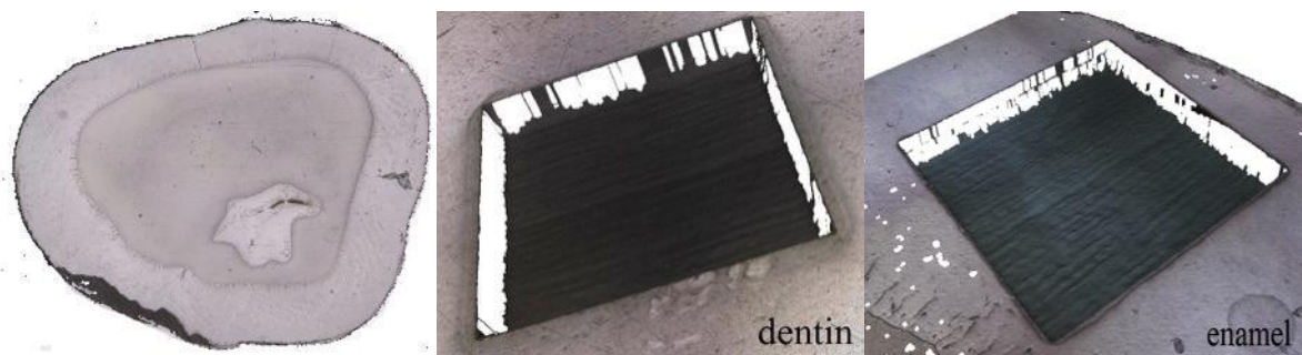
Figure 2. Optical microscopy imaging revealed no cracks or collateral damages after the ablation of dentin and enamel. Left: mirror-polished tooth slice prepared for ablation. Right: ablated enamel and dentin zones.
