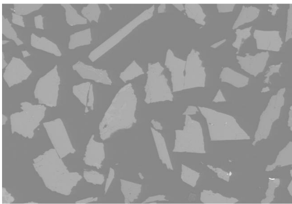
Figure 5 – BSE image (left) and elemental (Zr, Ce, Fe, Y) phase identification (right) of the DMS sink and float fraction produced using a heavy liquid with a SG of 2.75
