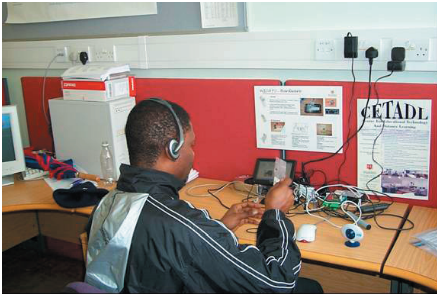
Figure 3. Interacting with objects tagged with RFID, using speech to input descriptions
