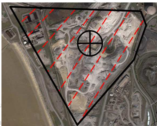
Figure 3. Wind roses identifying the cross sectioned area on the map as an area of most likely sources of PM 10 that contribute to high concentrations. [Plotted using data measured during campaign 18 April-16 May 2012, PM 10 units: \mu\text{g}/\text{m}^3 ]. Upper diagram shows the triangulation (using wind directions with PM 10 greater than the 90 th percentile) used to prescribe the source area and the lower diagram shows the aerial photograph of the area. [Little Warren (LW), Port Talbot Margam AURN (FS), Port Talbot Docks (DOCKS), Prince Street (PS), Twll-yn-y-Wall (Twll) and Dyffryn School (DS) sites].
