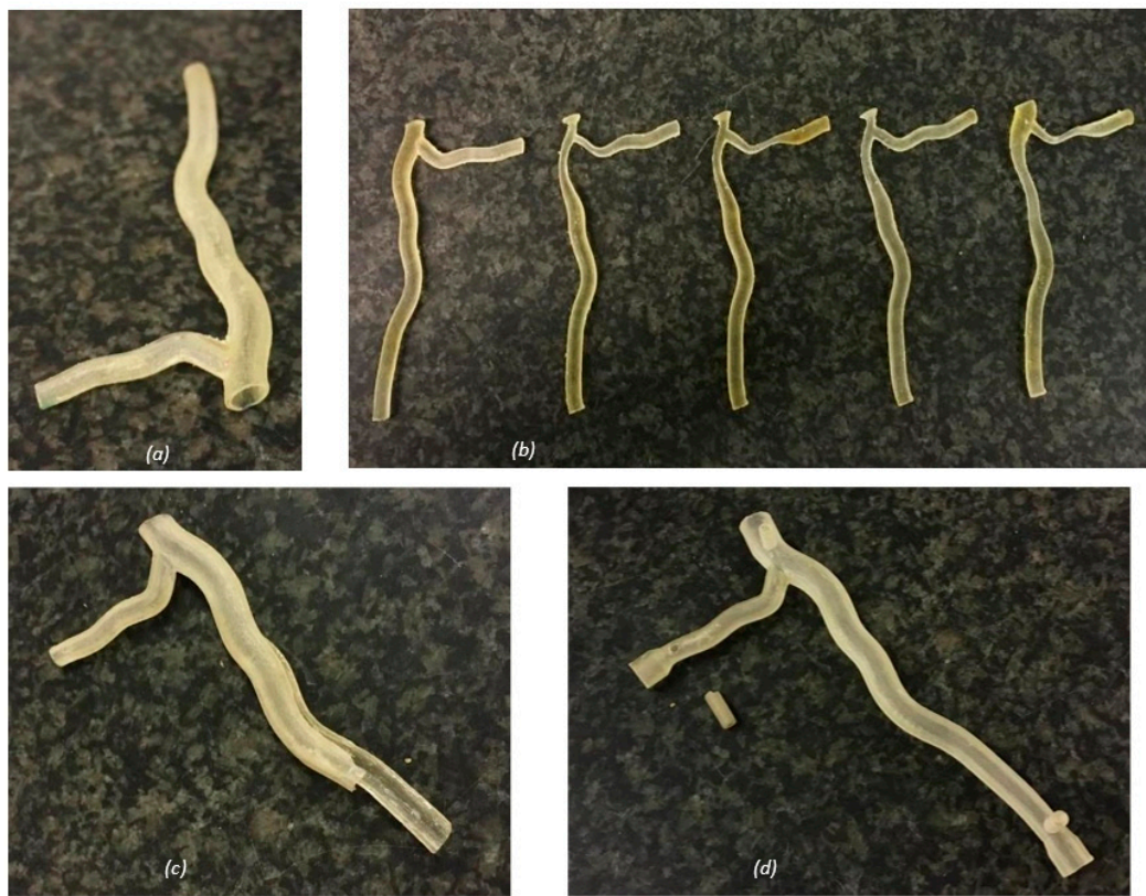
Figure 1. Printed resin models: (a) hollow healthy bifurcation; (b) anatomical solid models of the healthy and stenosed cases; (c) hollow artery model damage, with cracking along the length of the artery; and (d) hollow artery model with a connection via a small port (damaged during testing). Full design rationale and dimensions used to design the models are included in detail in Section 4.1.
