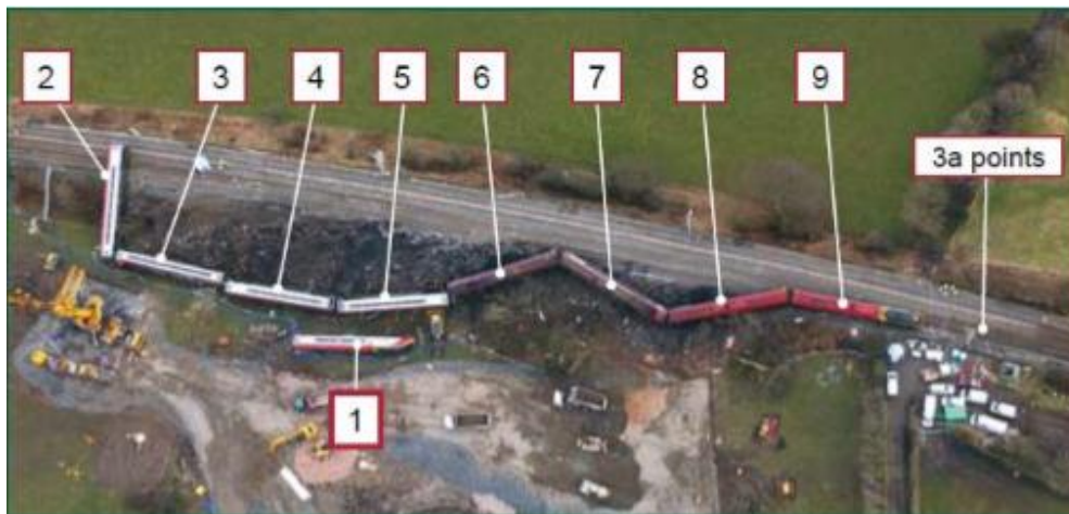
Fig.1: Aerial view of the derailed train from the Grayrigg derailment [6]
