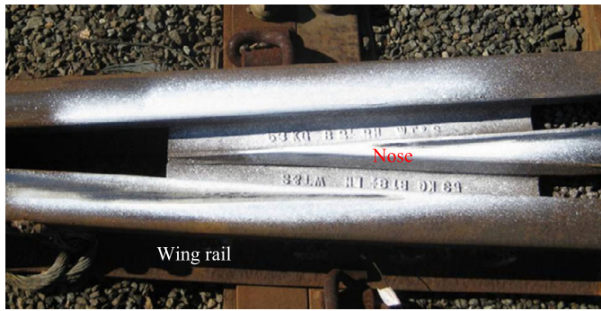
a) wheel traversing a v-crossing (white paint showing the contact band)
