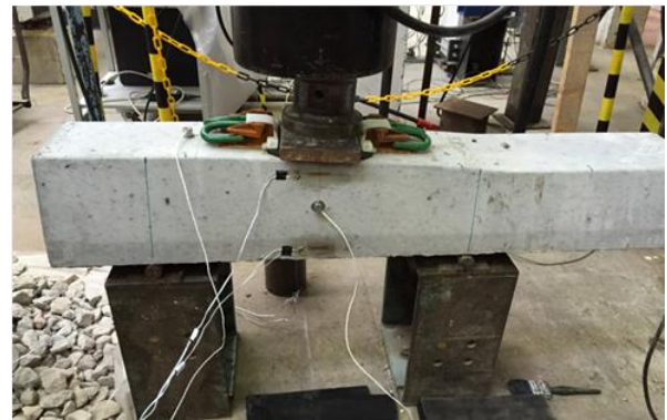
Figure 2. Standard type testing setup for performance benchmarking of sleeper capacity. Note that the type tests are normally used for quality assurance of materials and components.
