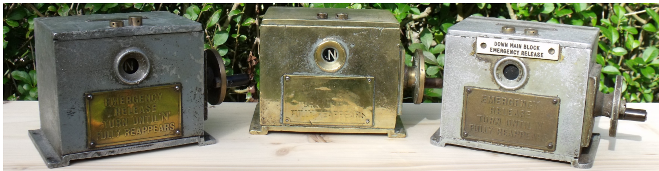
Figure 1. A set of railway lockout devices. The handles on the right-hand sides are wound to set the device. © Dr J M Saxton
