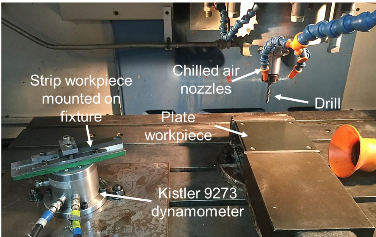
Figure 2. Experimental setup on Matsuura FX-5
