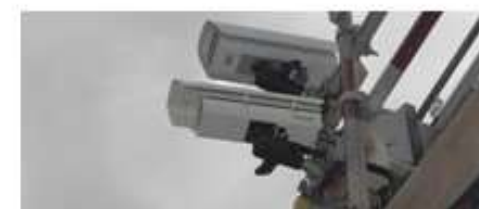
Figure S2: EDAR deployment at Greenwich Blackheath Hill as part of the UoB/UoL/KCL study. Left, the EDAR deployed on purpose-built scaffolding at the roadside, with the EDAR installed at 5 meters nearby rather than directly over the road and traffic flows. The same photograph also shows the PEMS vehicle approaching the reflector strips where EDAR exhaust emission measurements are made and (behind the scaffolding) the local air quality monitoring station. Right Top and Bottom, the two EDAR units (one for gaseous species, one for PM) and the speed and automatic number plate capture cameras, respectively.
